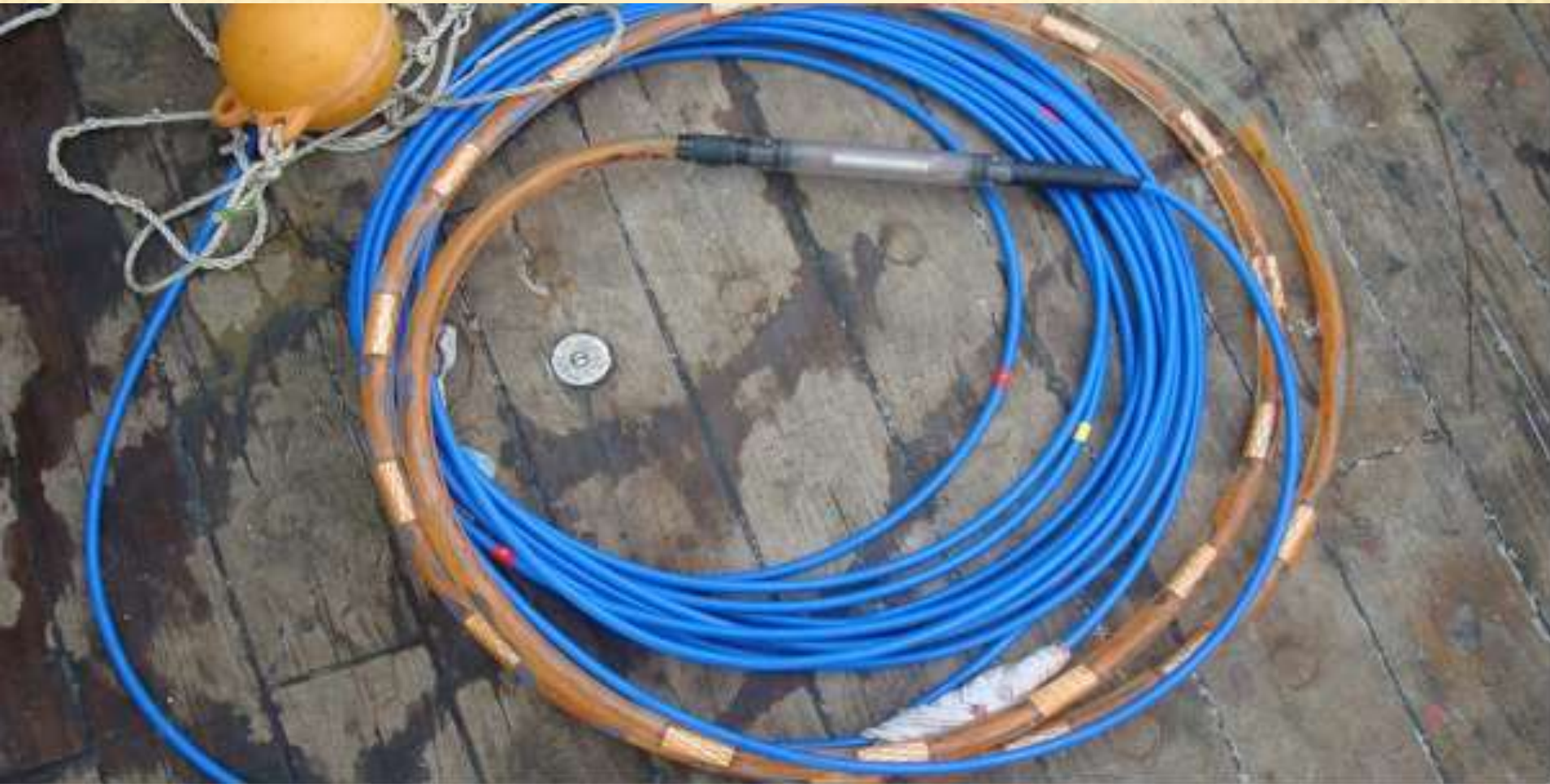
AN ARRAY OF HYDROPHONES ASSEMBLED IN FLUID FILLED CABLE
